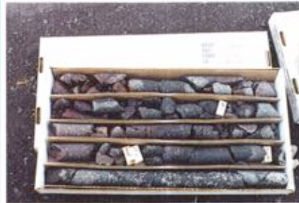
Figure 4-7 Petroleum Stained Core - BHC, 49" to 60"
