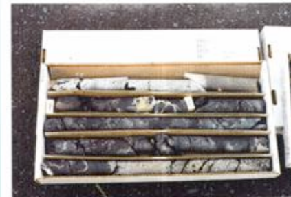
Figure 4-8 Petroleum Stained Core - BHC, 60" to 69"
