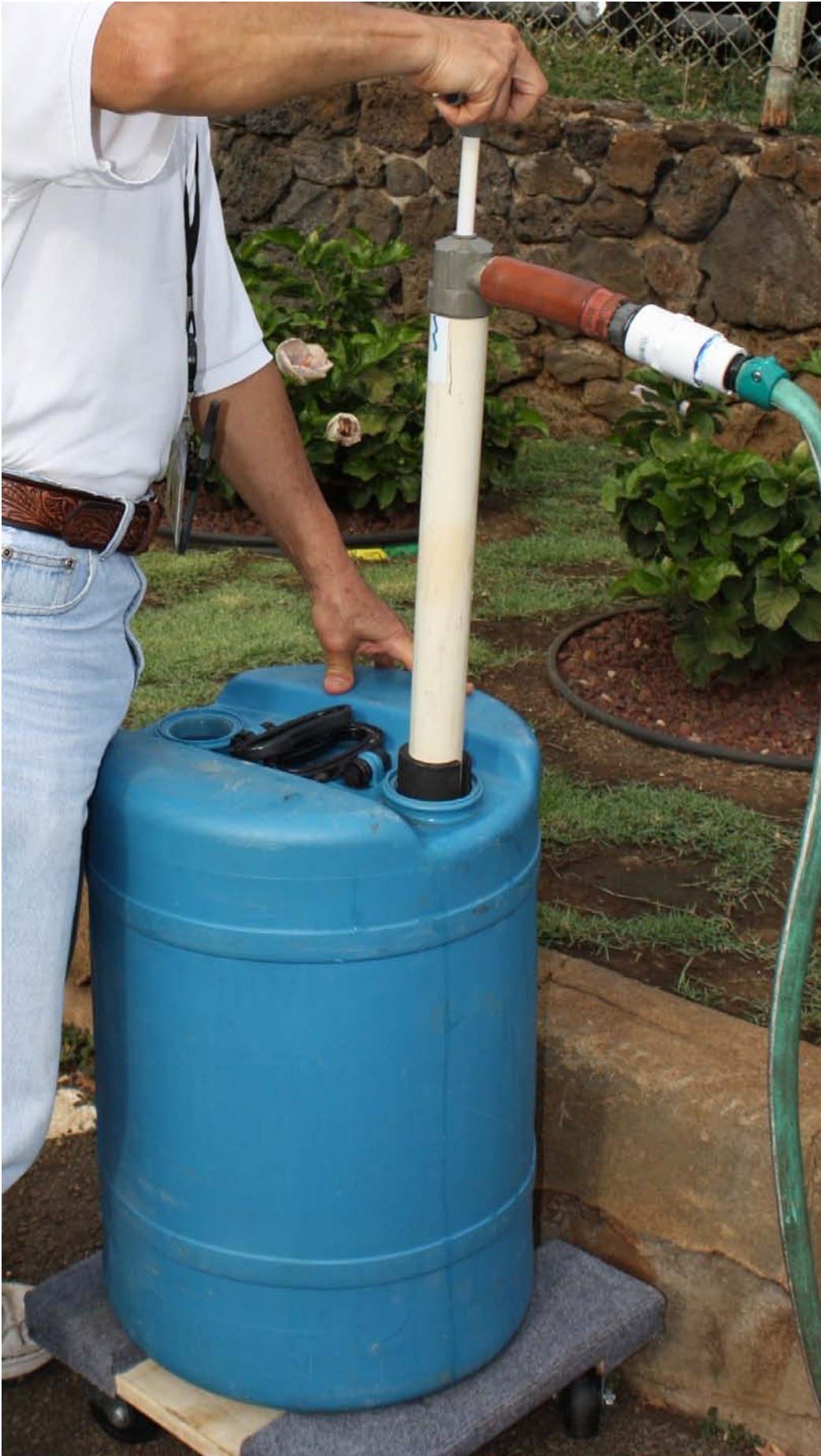
Hand pump used to manually extract water from a small drum
